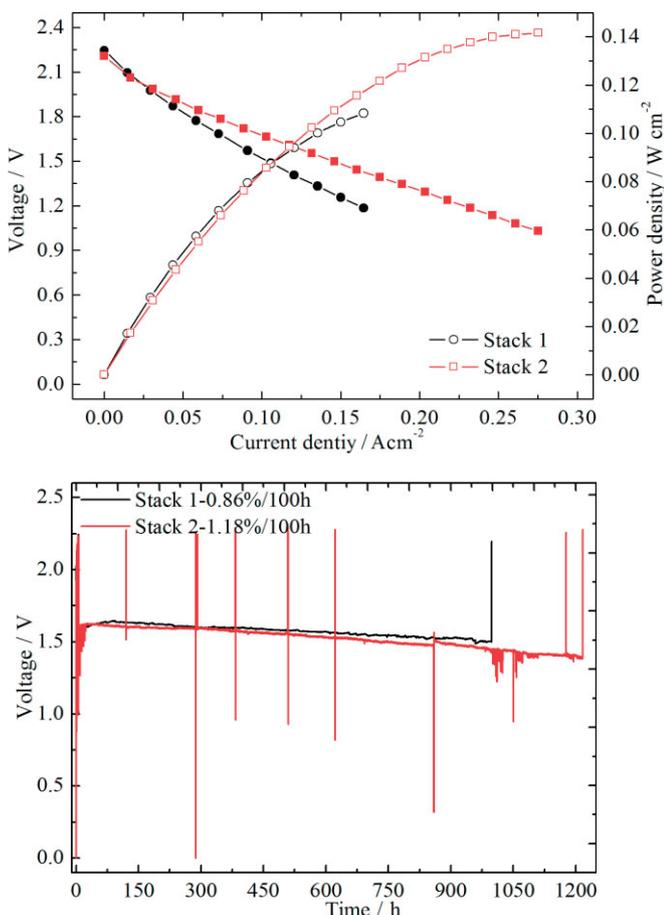
Fig. 2 Durability tests of stacks at 750 °C under 0.1 A cm<sup>-2</sup> discharging current.
