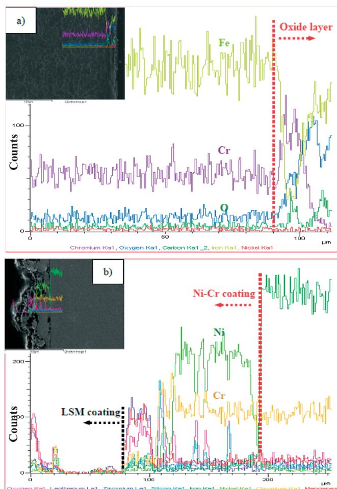
Fig. 13 EDS line on cathode side of interconnect: (a) uncoated interconnect B and (b) coated interconnect C.
