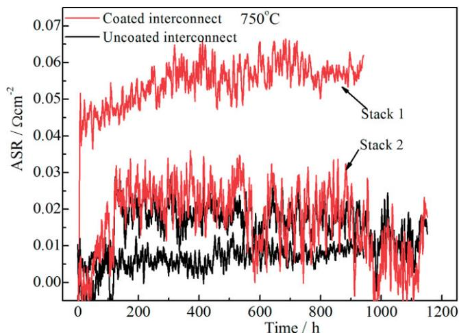
Fig. 5 The ASR of uncoated and coated interconnect under stack stable operation.
