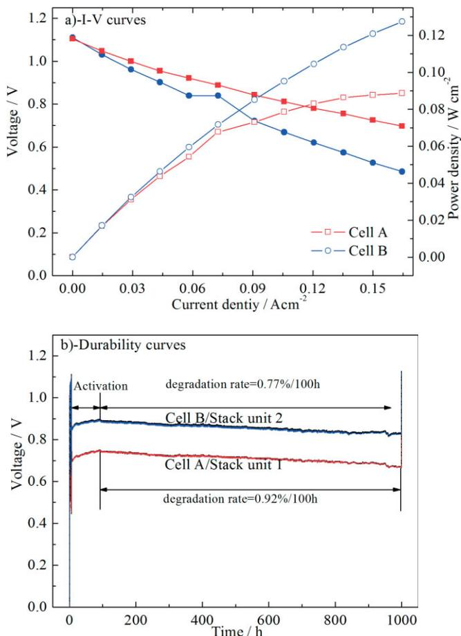
Fig. 3 *I-V* curves and durability curves of stack 1: (a) *I-V* curves and (b) durability curves.
