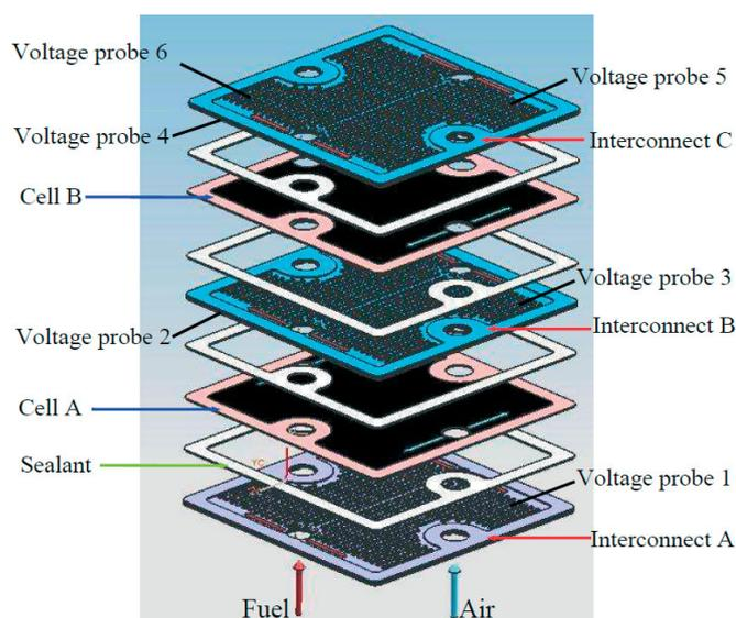
Fig. 1 Schematic diagram of stack assembly and probe locations in stack.
