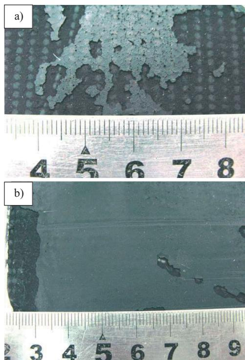
Fig. 10 Contact traces on cell cathode sides after testing in stack 2: (a) cathode side of cell A and (b) cathode side of cell B.
