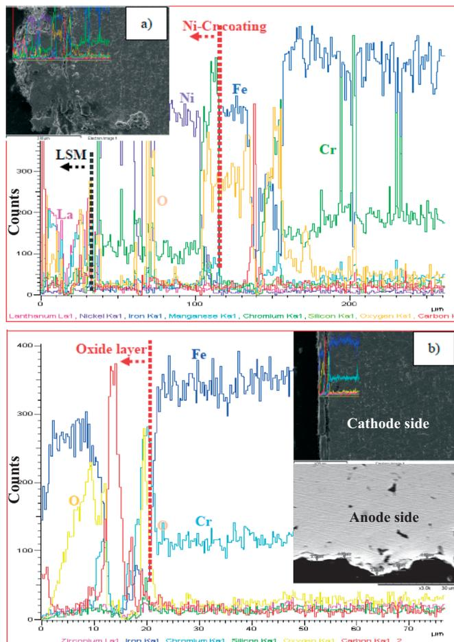
Fig. 6 The morphology and EDS line of interconnect: (a) coated and (b) uncoated.
